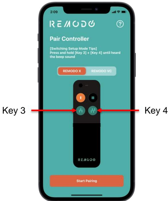
Each remote has a unique id (e.g. Remodo\_X\_setup\_00006) and the app will scan for this remote controller and indicate it to you.
